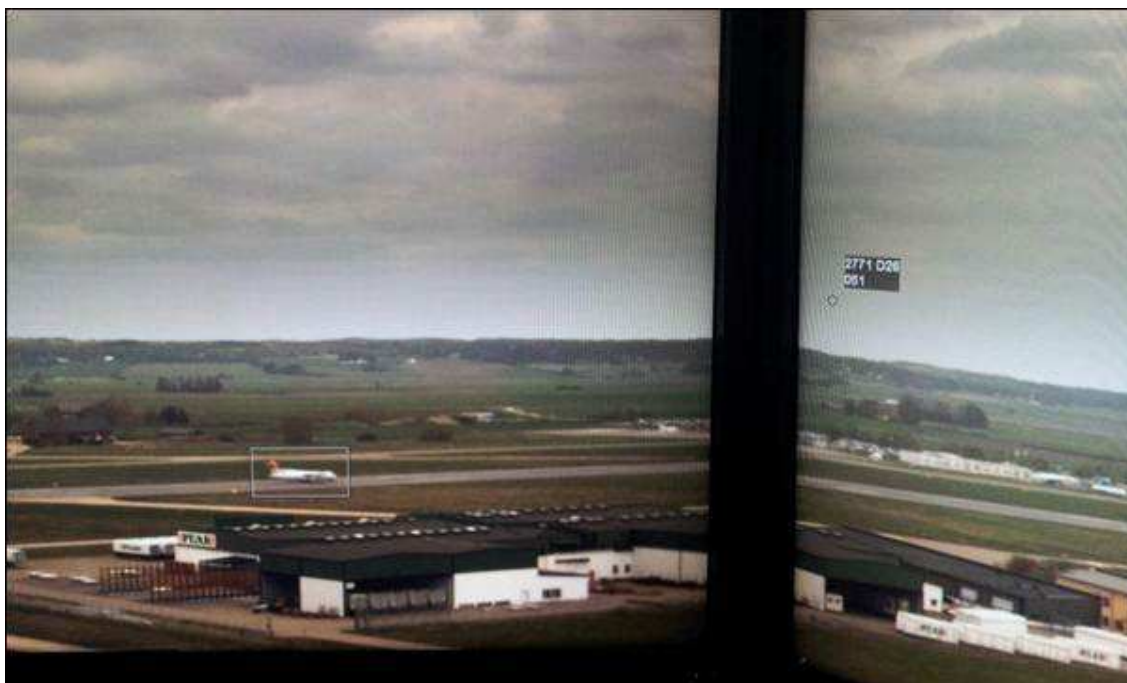
Figure 25 - Label overlays showing visual tracking (left) and radar tracking (right)
