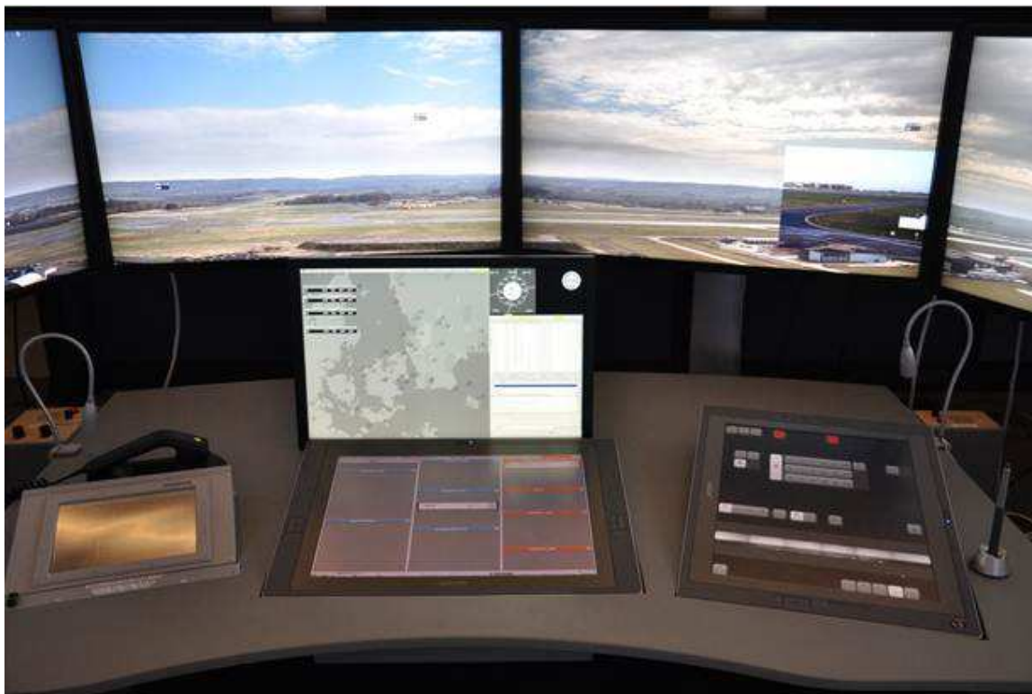
Figure 22 - CWP showing screens (top), e-strips (bottom centre), radar (centre middle), IDP (bottom right) and communications panel (bottom left)
